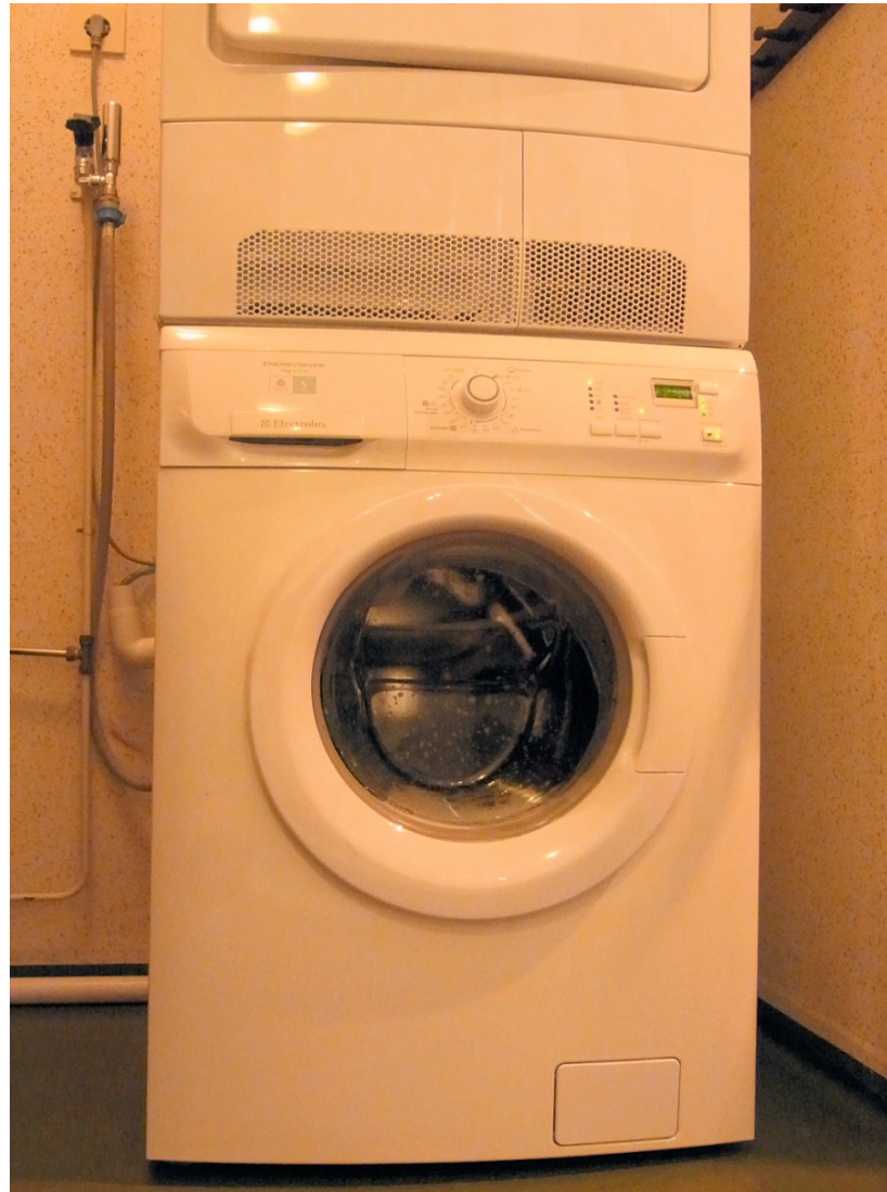
Washing machine with a brushless motor (RFI from interval-washing and spin-drier).
